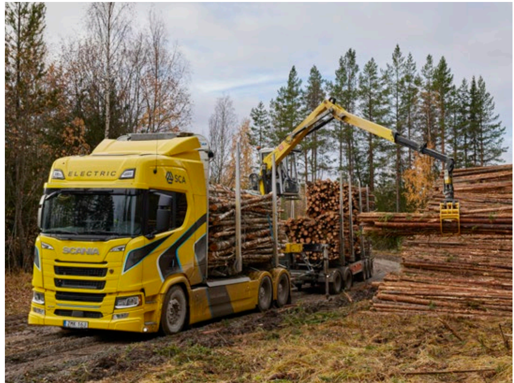
SCA's first electric timber truck, deployed in 2022, does not have a crane and is used for transports between a timber terminal and SCA's paper mill. The electric timber truck deployed in 2024 (above) features a crane and collects timber from the forest for transport to a timber terminal.
