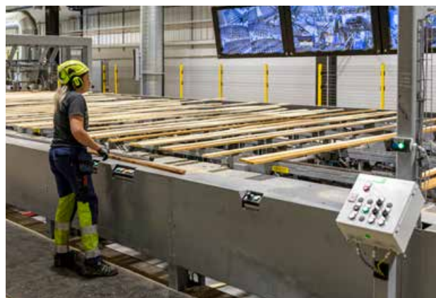
Bollsta sawmill's new CT scanner follows the progress of the log as it passes through the sawmill.
