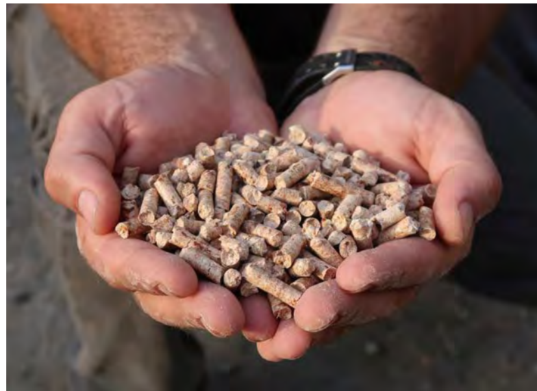
Sawdust from SCA's sawmills is made into pellets, which are sold to households and to major energy producers, and also used as fuel in SCA's own industry.
