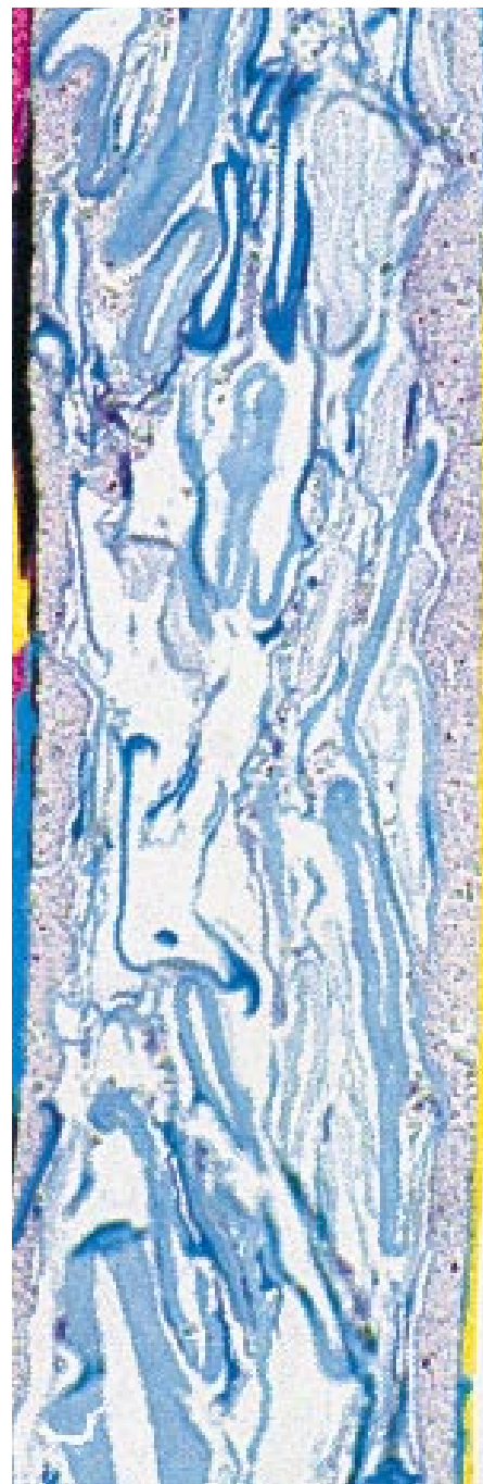
Cross-section of a 0.06-mm thick LWC paper. The photograph was taken using an optical microscope and illustrates the paper's complexity. The different colors show the distribution of mechanical (dark blue) and chemical pulp fibers (light blue), the coating layer (light red) and printing surface (cyan, magenta, yellow and black). Among other applications, the method is used to determine the strength and surface properties of the paper.
