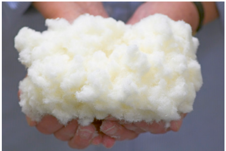
CTMP can be used in the manufacture of everything from cereal packets to liquid packaging board for products such as milk cartons.
