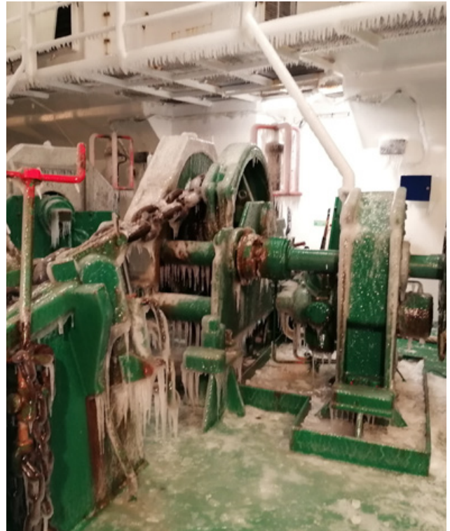
If it's windy and really cold, ice can form on the deck. This is important to pay attention to, because it can mean increased weight.
