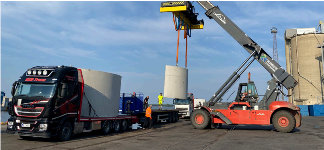
Concrete elements for wind power towers are loaded onto trucks in the port of Vaasa for onward transport to the construction site.
