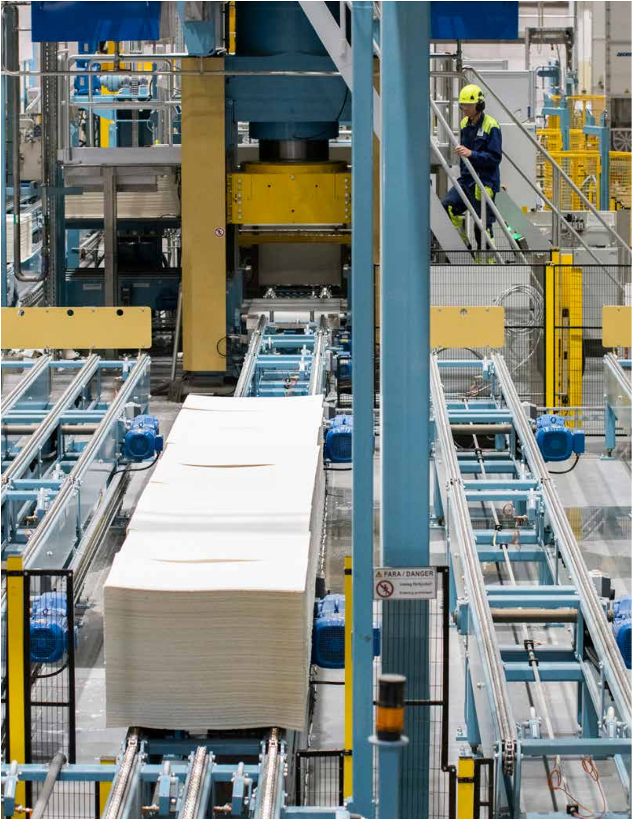
The pulp is cut into sheets, baled and packaged on the new drying line.
