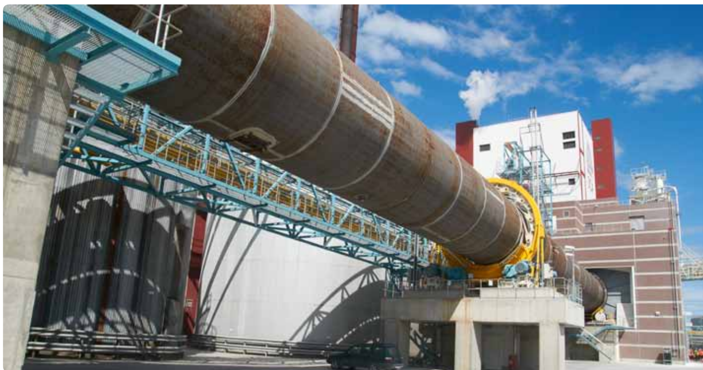
The installation of a biofuel-powered lime kiln at the Östrand pulp mill in Sweden reduced carbon dioxide emissions by 50,000 tons compared with using oil to power the old kilns.
