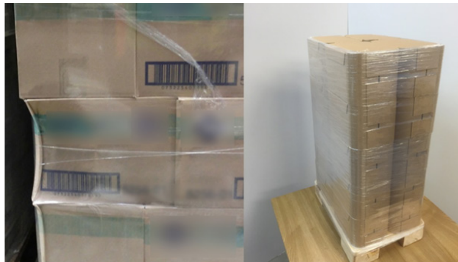
Fig. 8 Sharp angled corners can often be problematic in stretch wrapping with high tension (left hand side). The round corners distribute the load over a larger area and damaged corners are avoided (right hand side).
